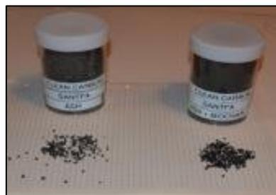
*Above – (L) 100% ash and (R) 80% ash + 20% Biochar. The poultry litter ash was granulated into a flowable and low dust product suitable for application with cropping equipment.*
